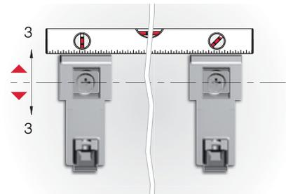
Recommended fixing countersunk screw type - head Ø 5 mm max.
